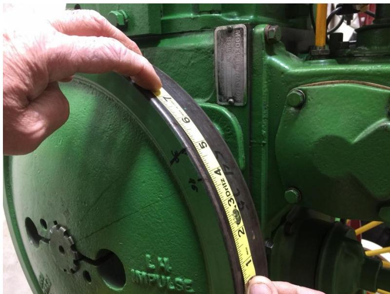
So..... if you want to set the timing for 30 degrees BTDC, place a mark on the flywheel at 4.5" CCW from TDC mark. Connect the timing light and determine the current timing relative to the TDC mark on the transmission cover. It should be around  $35^{\circ}$  on early tractors.
